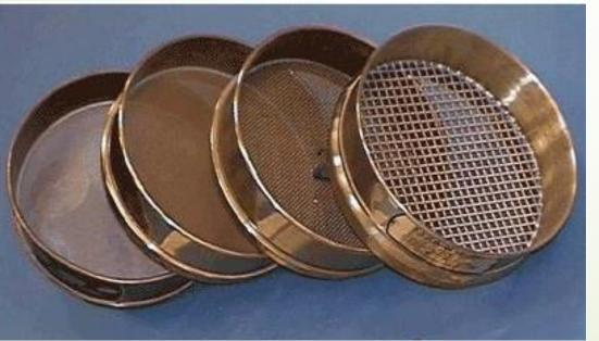
These precision screen openings are made to only allow a specific size particle to pass through. The desired pans are stacked on top of one another with the courser screens on top.
