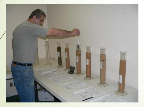
Determining the amount of silts and clays for Soil Classification is a very different approach and uses a wet method. A wet method is needed for silts and clays due to the fact of their difficulty in shaking through the sieves.
