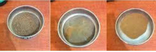
The soil that is retained on each screen is then weighed.
