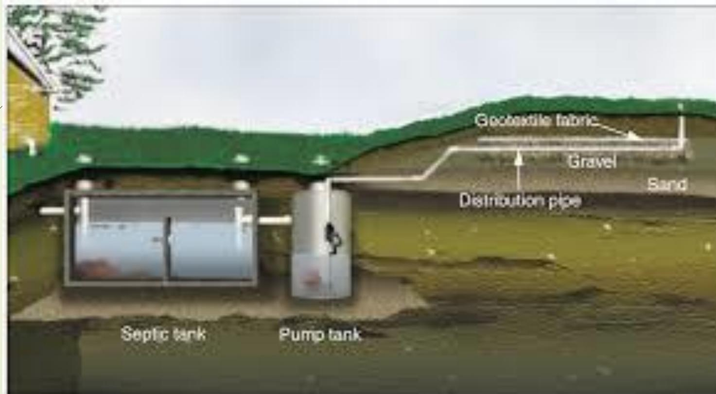
Figure 1: A mounded system for distributing treated wastewater to the soil.
