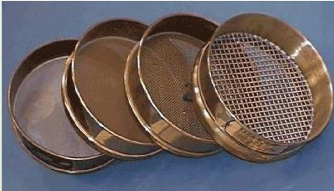
These precision screen openings are made to only allow a specific size particle to pass through.
