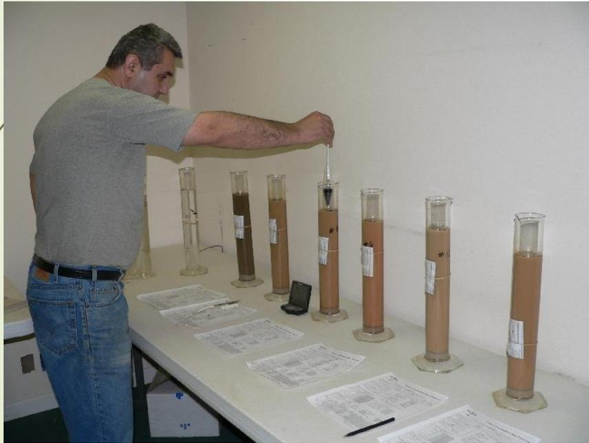
Determining the amount of silts and clays for Soil Classification is a very different approach and uses a wet method.
